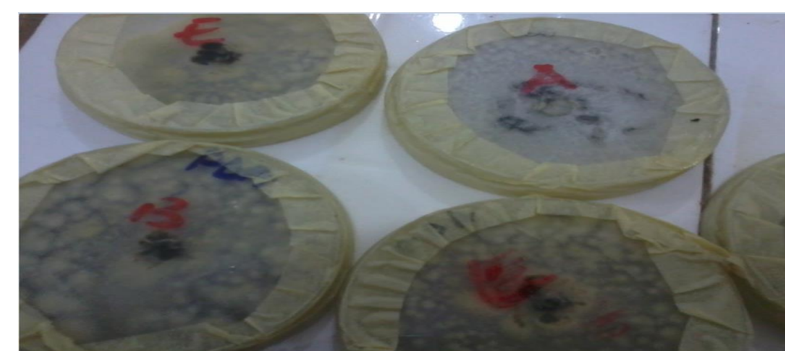
FIGURE 1: SCREENING FOR CELLULOLYTIC FUNGI ON CARBOXYL METHYL CELLULOSE AGAR PLATE.
